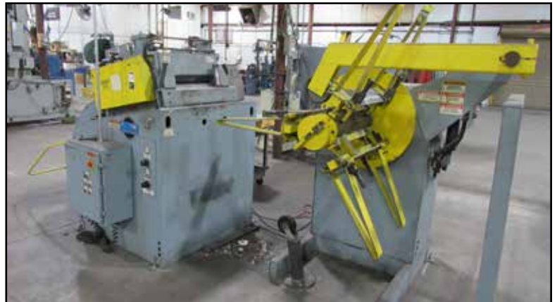
COE FEED LINE & UNCOILER
