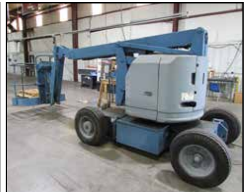
GENIE ELECTRIC BOOM MANLIFT
