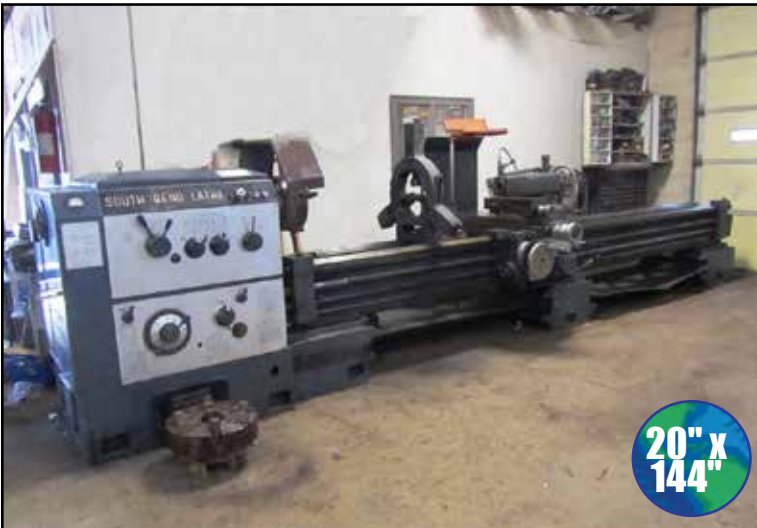
SOUTHBEND 22" SWING X 156" MAX. CENTERS HEAVY DUTY ENGINE LATHE
