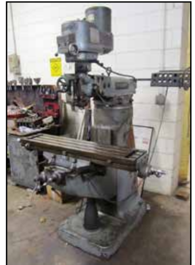
BRIDGEPORT SERIES 1 VARIABLE SPEED MILLING MACHINE
