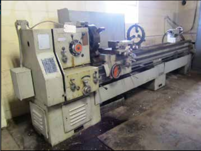
LAMCO 22" SWING X 120" MAX CENTERS ENGINE LATHE
