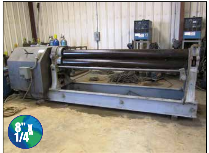
8' X 1/4" CAPACITY PLATE BENDING ROLL
