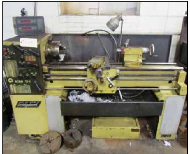
BRIDGEPORT ROMI 14" SWING X 40" CENTERS TOOL ROOM ENGINE LATHE
