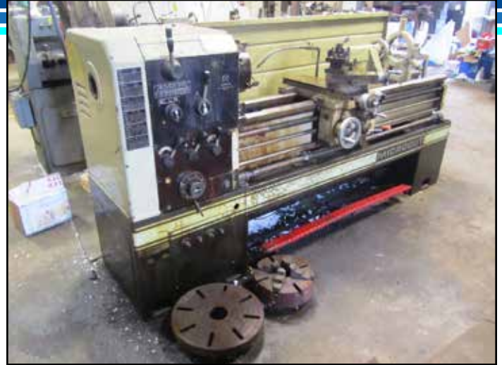
20" SWING X 56" MAX. CENTERS TOOL ROOM ENGINE LATHE
