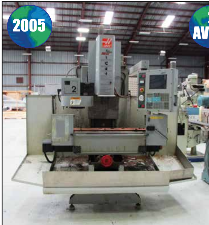
(2) HAAS TM2 3-AXIS CNC TOOLROOM MACHINING CENTERS / MILLS
