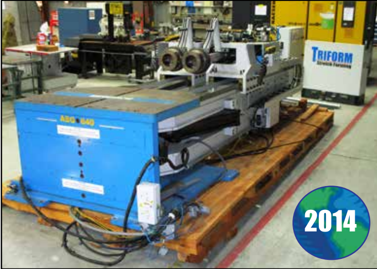
BECKWOOD TRIFORM SF20T-240 20 TON X 240" HYDRAULIC EXTRUSION STRETCH FORMING MACHINE
