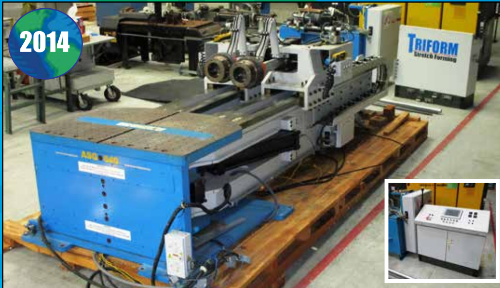
BECKWOOD TRIFORM SF20T-240 20 TON X 240" HYDRAULIC EXTRUSION STRETCH FORMING MACHINE
