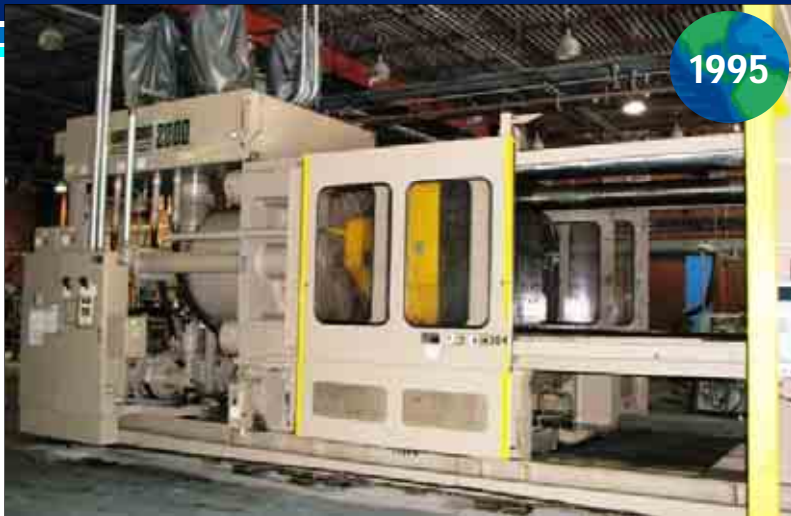
VAN DORN 2000 TON 260 OZ. MODEL 2000 HRS 260 FLP WIDE PLATTEN MOLDING MACHINE WITH CONAIR SEPRO SERVO ROBOT
