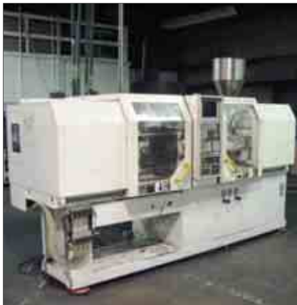
DEMAG 25 TON x 1.82 Oz. MODEL ERGOTECH 25-120 MOLDING MACHINE
