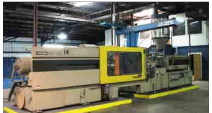
TOSHIBA 720 TON x 120 Oz. MODEL ISE710 MOLDING MACHINE
