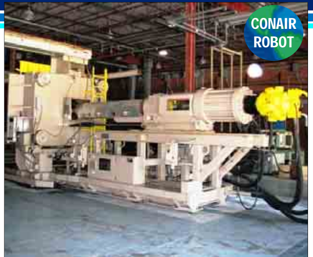
VAN DORN 2000 TON 260 OZ. MODEL 2000 HRS 260 FLP WIDE PLATTEN MOLDING MACHINE WITH CONAIR SEPRO SERVO ROBOT
