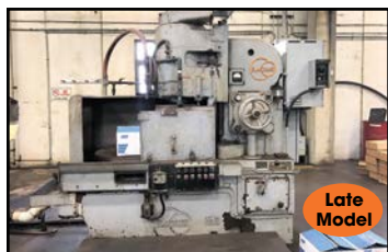
BLANCHARD # 18-36 VERTICAL ROTARY GRINDER
