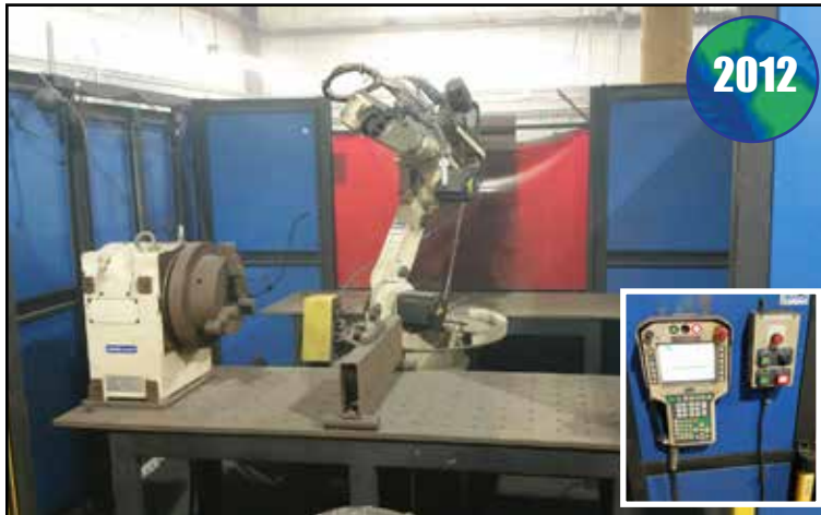
FUSHION ARC ROBOT WELDING CELL
