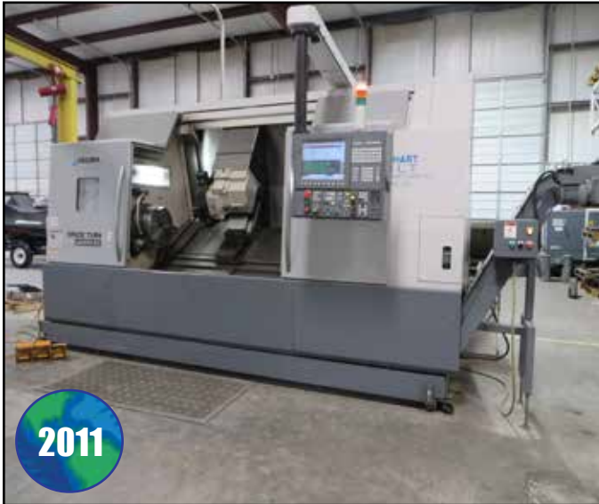
OKUMA SPACE TURN LB4000EX - MY C1500 CNC TURNING CENTER WITH Y-AXIS, MILLING & C-AXIS
