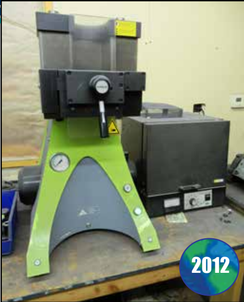
REGO-FIX POWRGRIP PGU9006 POWER TOOL SETTER
