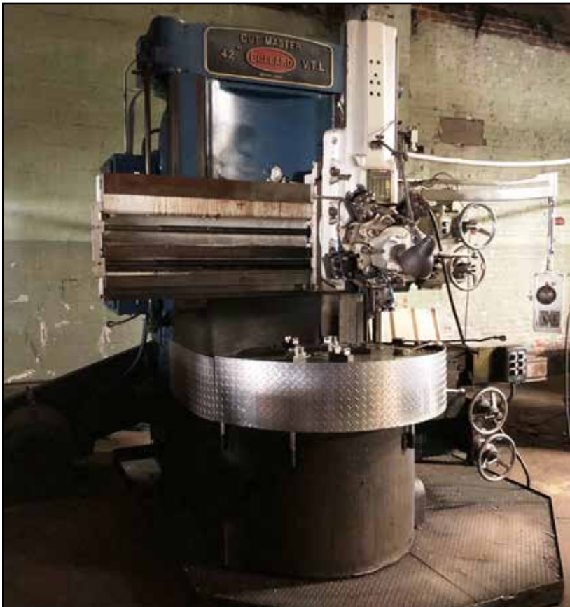
BULLARD CUT MASTER 42" VERTICAL TURRET LATHE
