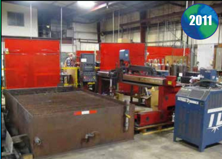
KOIKE ARONSON 6' X 10' CNC PLASMA CUTTING MACHINE
