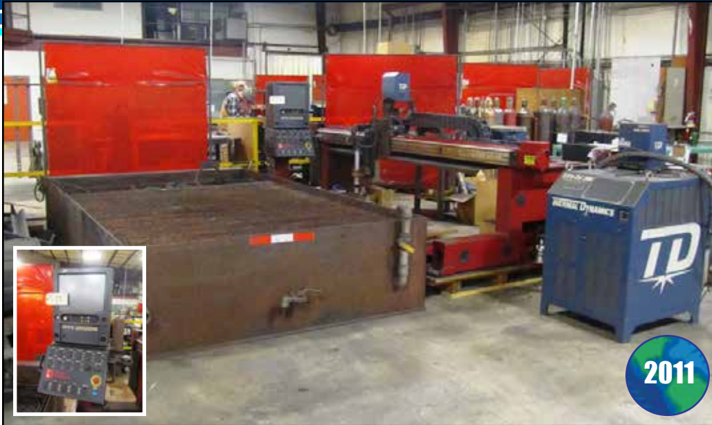
KOIKE ARONSON 6' X 10' CNC PLASMA CUTTING MACHINE
